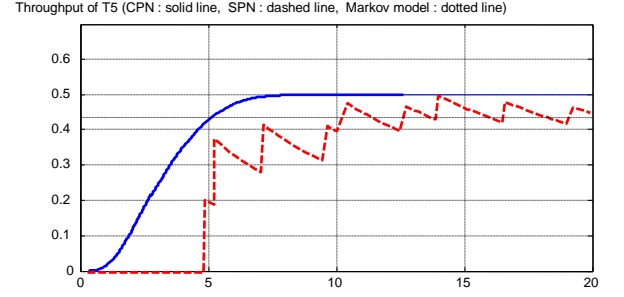
Fig. 2. Throughput evolution X_{atc}(t) and X_{ats}(t) of CPN (solid line) and SPN (dashed line) in function of time, for example of fig. 1.
